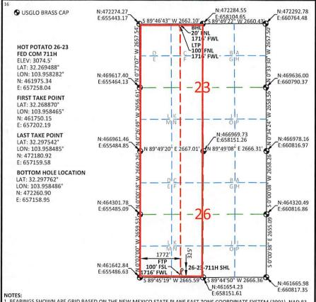
1. BEARINGS SHOWN ARE GRID BASED ON THE NEW MEXICO STATE PLANE EAST ZONE COORDINATE SYSTEM (3001), NAD 83 (2011), BASED FROM GPS OBSERVATIONS, OCCUPYING A WHS CONTROL POINT (5/8" REBAR), LOCATED AT NORTH: 456034.443, EAST: 653560.641, ELEVATION: 3101.4, DETERMINED BY AN OPUS SOLUTION ON MOVEMBER 9TH, 2019.
