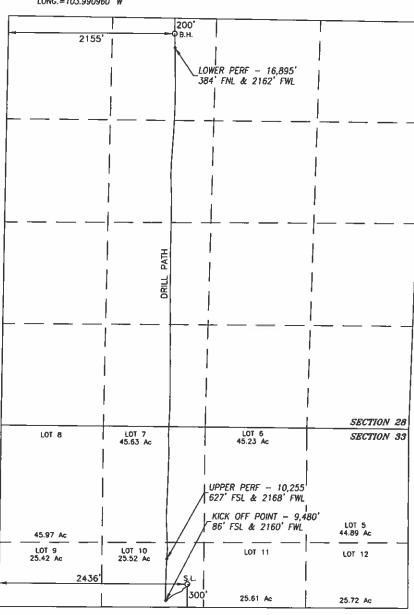
NAD 83 NME <u>SURFACE LOCATION</u> Y=364249.5 N X=647661.3 E LAI.=32.000938° N LONG.=103.990338° W BOREPATH SHOWN HEREON IS BASED ON DIRECTIONAL SURVEY REPORT PROVIDED BY COG OPERATING, LLC FOR THE LITTLEFIELD 33 FEDERAL COM #705th SUPPLIED TO HARCROW SURVEYING, LLC ON JUNE 5, 2019
