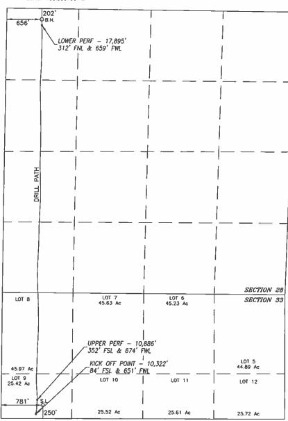
NAD 83 NME SURFACE LOCATION Y=364195.2 N X=646006.3 E LAT.=32.000803' N LONG. = 103.995677' W BOREPATH SHOWN HEREON IS BASED ON DIRECTIONAL SURVEY REPORT PROVIDED BY COG OPERATING, LLC FOR THE LITTLEFIELD 33 FEDERAL COM \$808H SUPPLIED TO HARCROW SURVEYING, LLC ON JUNE 4, 2019
