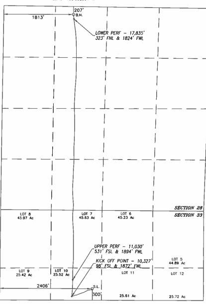
NAD 83 NME SURFACE LOCATION Y=364249.4 N X=647631.3 E LAT. = 32.000938' N LONG.=103.990434° W BOREPATH SHOWN HEREON IS BASED ON DIRECTIONAL SURVEY REPORT PROVIDED BY COG OPERATING, LLC FOR THE LITTLEFIELD SO FEDERAL COM #806H SUPPLIED TO HARCROW SURVEYING, LLC ON JUNE 5, 2019
