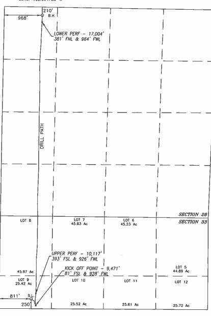
NAD 83 NME <u>SURFACE LOCATION</u> Y=364195.2 N X=646036.3 E LAT.=32.000803\* N LONG.=103.995580\* W BOREPATH SHOWN HEREON IS BASED ON DIRECTIONAL SURVEY REPORT PROVIDED BY COG OPERATING, LLC FOR THE LITTLEFIELD 33 FEDERAL COM #70TH SUPPLIED TO HARCROW SURVEYING, LLC ON MAY 23, 2019
