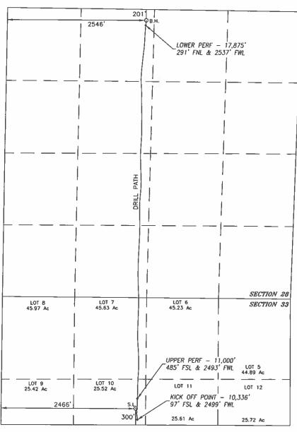
NAD 83 NME <u>SURFACE LOCATION</u> Y=364249.5 N X=647691.2 E LAT.=32.000938 N LONG.=103.990241 W BOREPATH SHOWN HEREON IS BASED ON DIRECTIONAL SURVEY REPORT PROVIDED BY COG OPERATING, LLC FOR THE LITTLEFIELD 33 FEDERAL COM #805H SUPPLIED TO HARCROW SURVEYING, LLC ON JUNE 28, 2019
