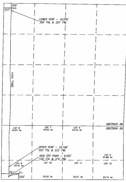
NAD 83 NME SURFACE LOCATION Y=364195.1 N X=645976.3 E LAT.=32.000803' N LONG. = 103.995774' W BOREPATH SHOWN HEREON IS EASED ON DIRECTIONAL SURVEY REPORT PROVIDED BY COG OPERATING, ILC FOR THE LITTLEFIELD 3S FEDERAL COM \$708H SUPPLIED TO HARCROW SURVEYING, ILC ON JUNE 5, 2019
