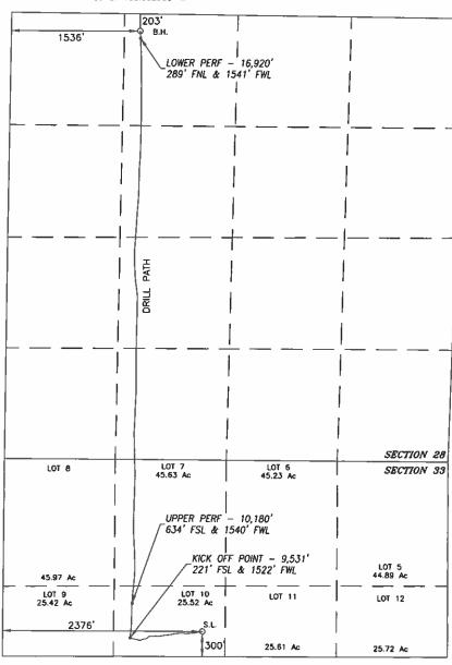
NAD 83 NME SURFACE LOCATION Y=364249.3 N X=647601.2 E LAT.=32.000938" N LONG.=103.990531' W BOREPATH SHOWN HEREON IS BASED ON DIRECTIONAL SURVEY REPORT PROVIDED BY COG OPERATING, LLC FOR THE LITTLEFIELD 33 FEBERAL COM #706H SUPPLIED TO HARCROW SURVEYING, LLC ON MAY 23, 2019
