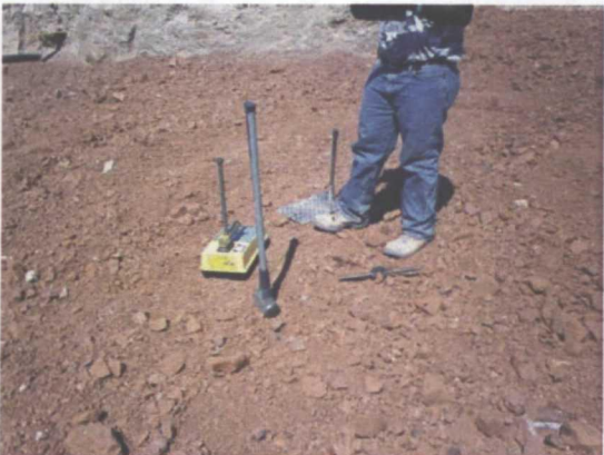
clay compaction test on the south side excavation 6/23/2011
