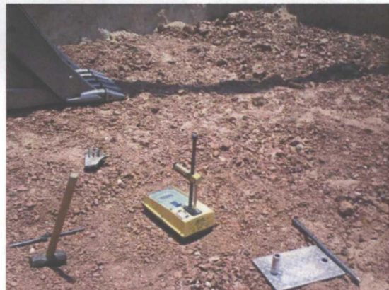
clay compaction test on the north side excavation 6/13/2011
