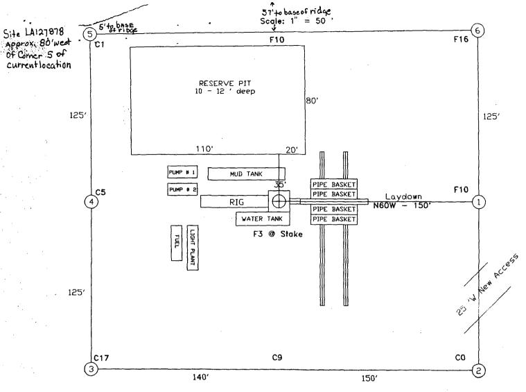
50' Construction Buffer on all corners except 2, 3, & 5. Side 2-3 will be 1:1 cutslope outside stakes. Corner 5 will be rounded inside the stake. Drainage berm will be started at corner 5 stake.
