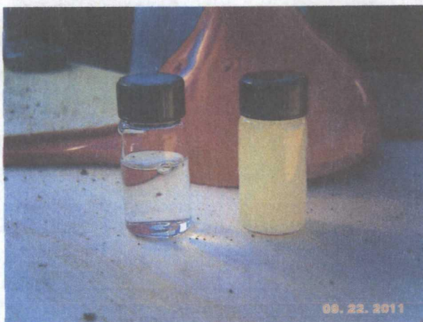
Field TPH results for above soil pile: TPH> Instrument range>6000 ppm Re-ran 10:1 dilution TPH = 25,720 ppm Chlorides = 544 ppm & 884 ppm.
