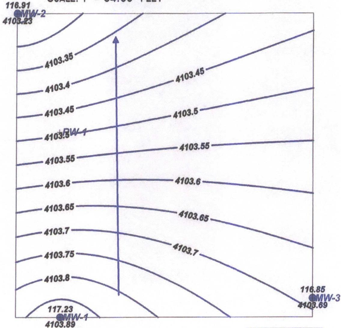
GROUNDWATER FLOW DIRECTION INDICATED BY BLUE FLOW LINES
