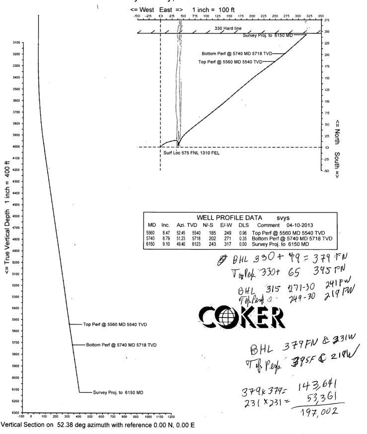
Vertical Section on 52.38 deg azimuth with reference 0.00 N, 0.00 E
