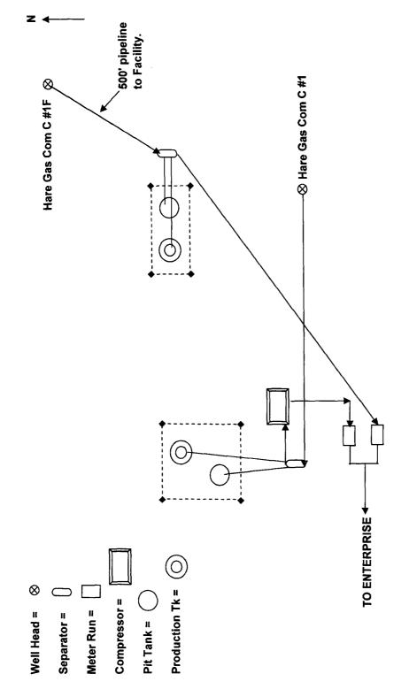
Note: The Hare Gas Com C #1F meter run is only 60' from the compressor suction. Also there is a lot of restriction for the PM Plunger system because of the high LP.
