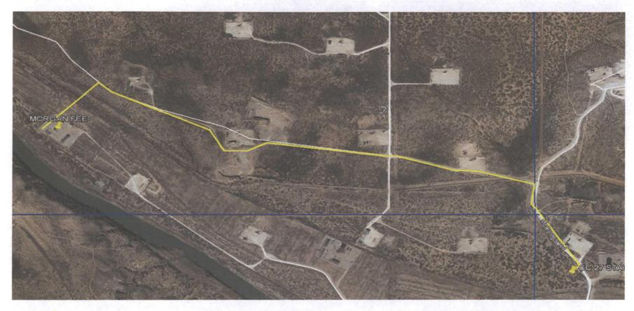
4" FP301 surface flowline will be routed from Cedar Canyon 27 State Com 4H well to Morgan fee battery. Length of flow line is estimate to be 6,500 ft. The flowline is laid on fee surface.
