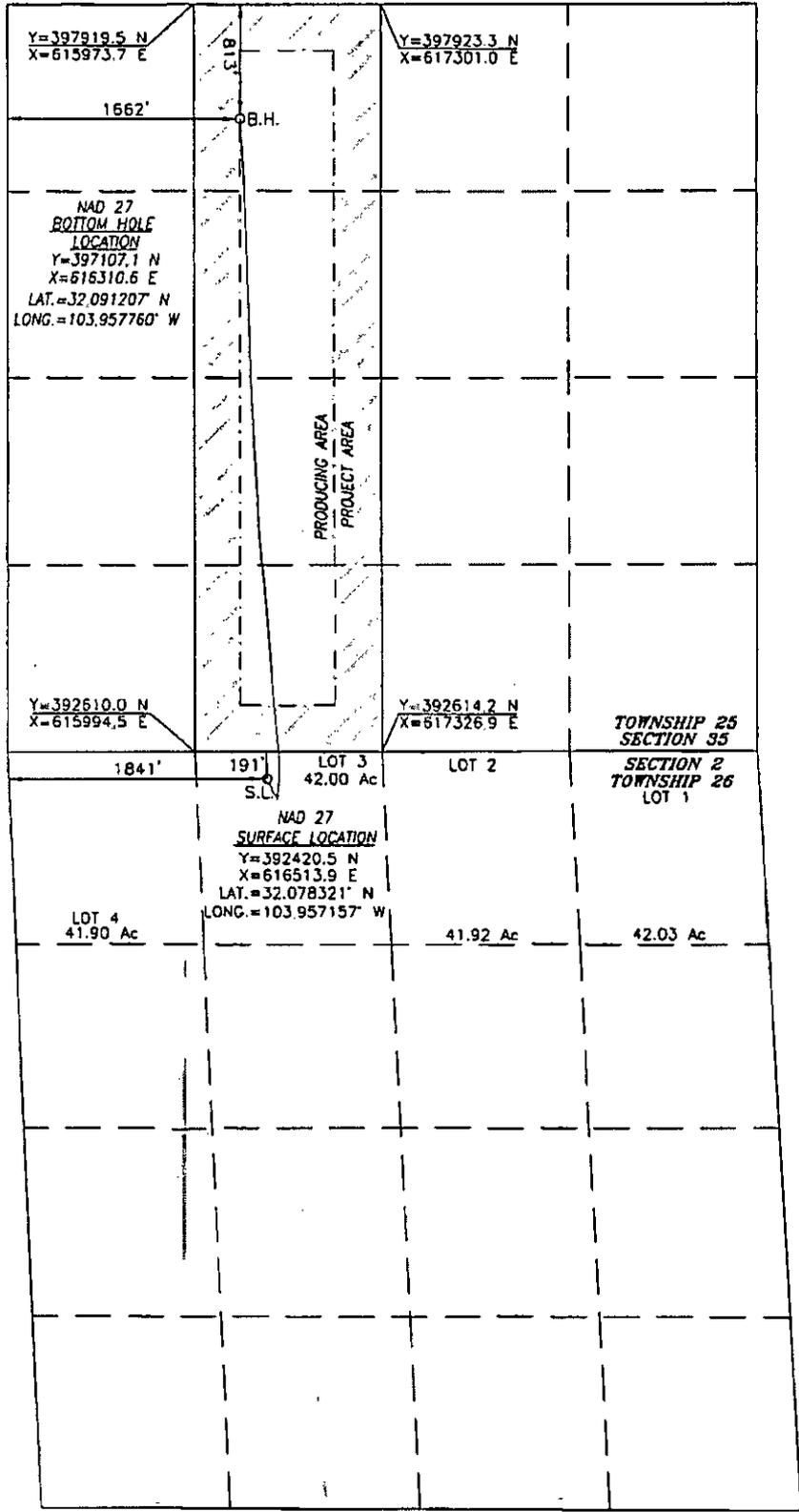
BOREPATH SHOWN HEREON IS BASED ON A DIRECTIONAL SURVEY REPORT PROVIDED BY TDS FOR THE OSPREY EO STATE COM #1H ON SEPTEMBER 23, 2014.
