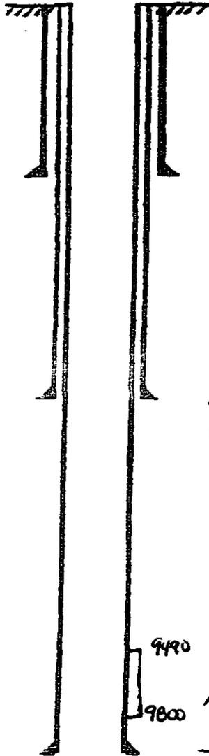
$13\frac{3}{8}$ " casing set at 1050' with 1000 SX of \_\_\_\_\_
