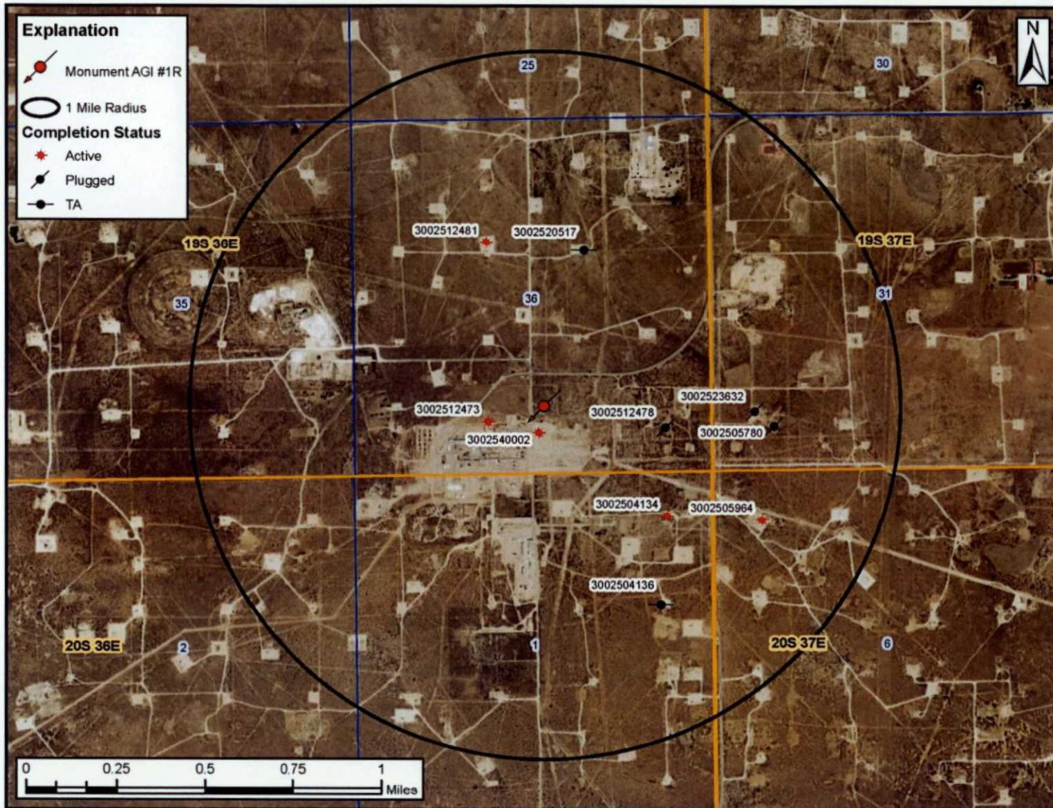
**Figure A2:** Oil and Gas Wells Penetrating the Injection Zone within One Mile of Proposed AGI #1R
