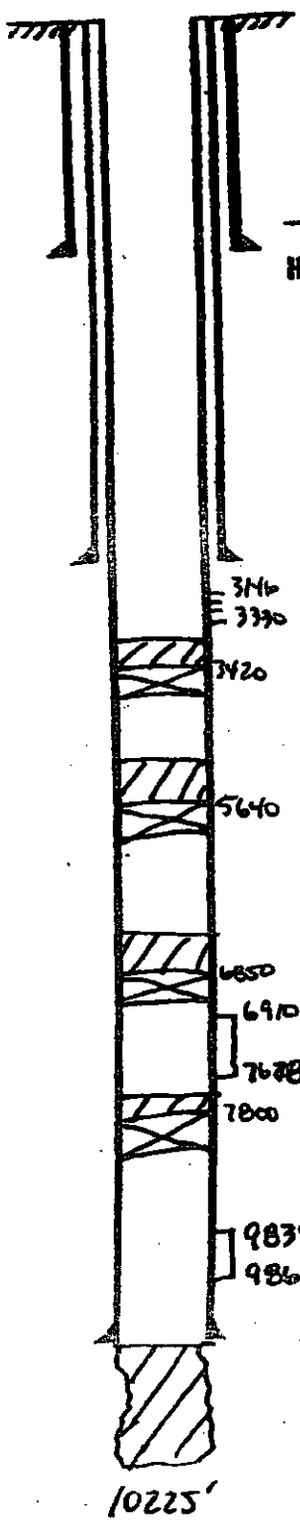
$13\frac{3}{8}$ " casing set at 187' with 200 sx of \_\_\_\_\_ cement
