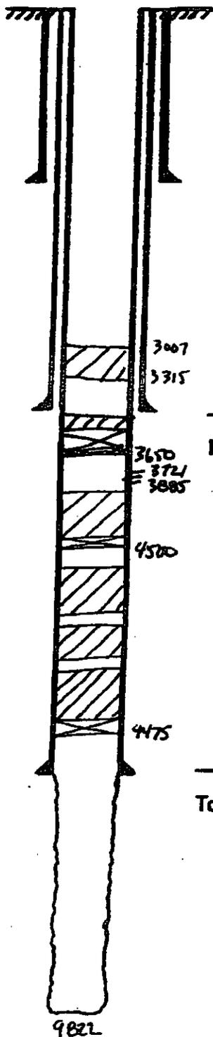
13 7/8" casing set at 302' with 300 sx of \_\_\_\_\_
