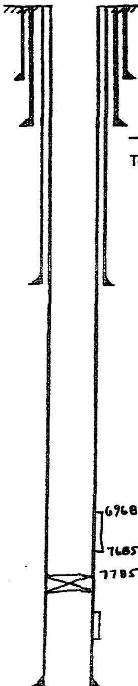
16 " casing set at 169 ' with 300 sx of \_\_\_\_\_ cement
