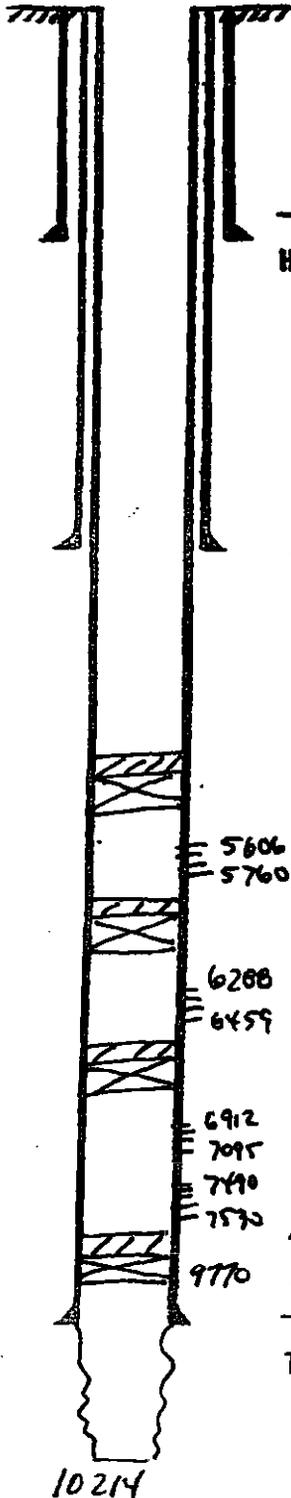
$13\frac{3}{8}$  " casing set at 997 ' with 750 sx of \_\_\_\_\_ ce
