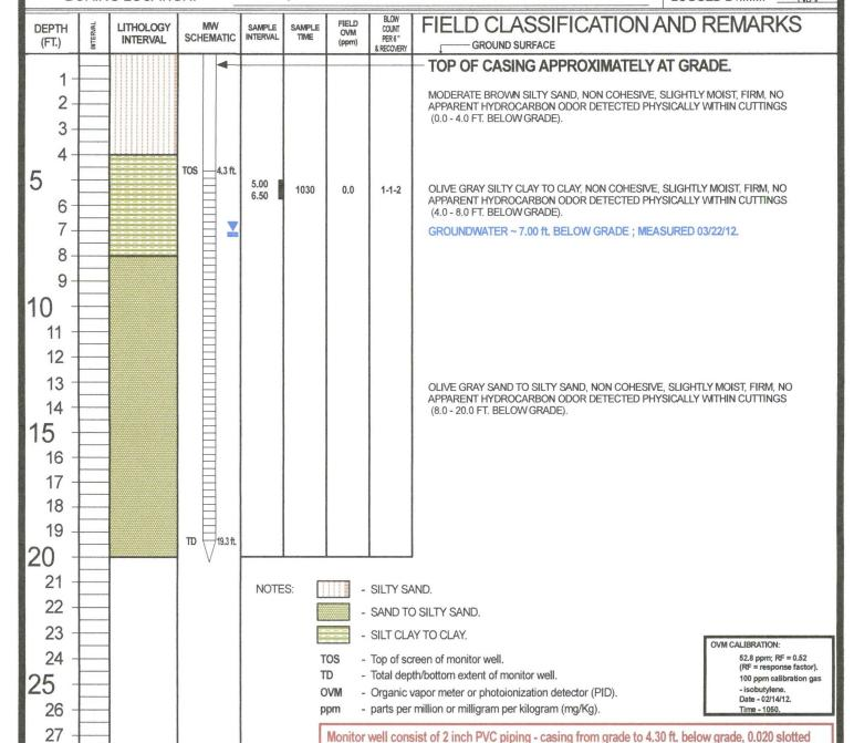
screen between 4.30 to 19.30 ft, below grade, sand packed annular to 2.0 ft, below grade, bentonite
