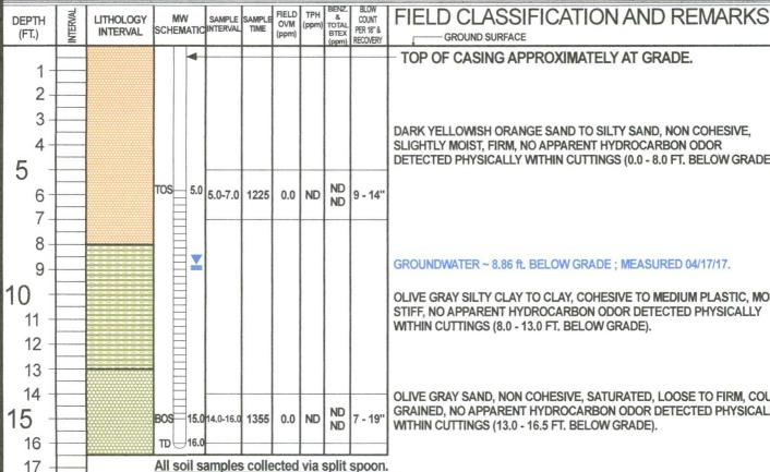
DARK YELLOWISH ORANGE SAND TO SILTY SAND, NON COHESIVE. SLIGHTLY MOIST, FIRM, NO APPARENT HYDROCARBON ODOR DETECTED PHYSICALLY WITHIN CUTTINGS (0.0 - 8.0 FT. BELOW GRADE).
