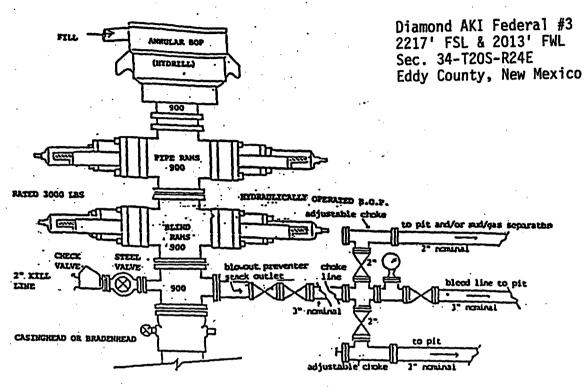
typical choke manifold assumby (or 1% rated working pressure service-surface installation
