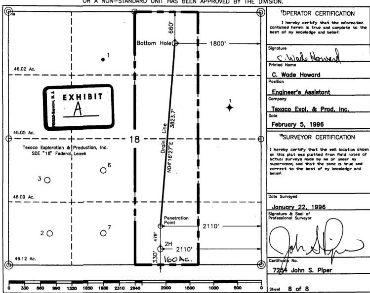
O = Staked Location • = Producing Well = Injection Well • = Water Supply Well • = Plugged & Abandon Well O = Found /4 Section Corner, 1" Iron Pipe & GLO B.C. = Found Section Corner, 2 or 3" Iron Pipe & GLO B.C.
