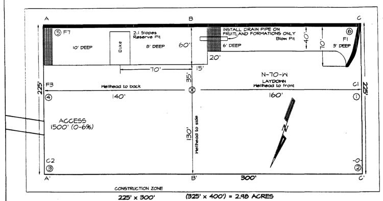
Reserve Pit Dike: to be 8' above Deep side (overflow - 3' wide and 1' above shallow side). Blow Pit: overflow pipe halfway between top and bottom and to extend over plastic liner and into blow p
