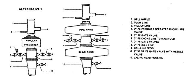
NOTE: THE DRILLING SPOOL MAY BE LOCATED BELOW BOTH SETS OF RAMS IF A DOUBLE PREVENTER IS USED AND IT DOES NOT HAVE SUITABLE OUTLETS BETWEEN RAMS
