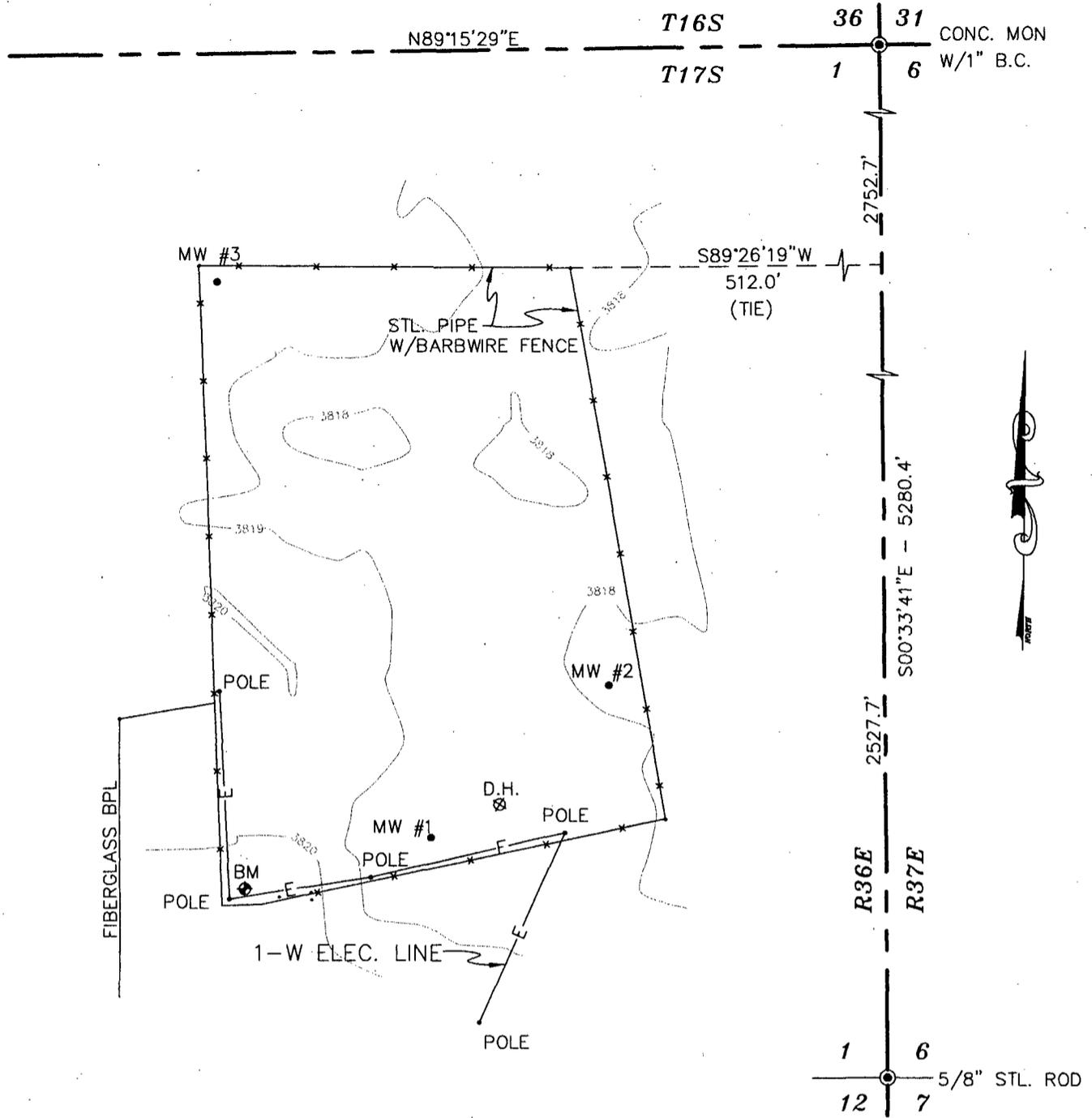
NOTE: BEARINGS SHOWN HEREON ARE MERCATOR GRID AND CONFORM TO THE NEW MEXICO COORDINATE SYSTEM "NEW MEXICO EAST ZONE" NORTH AMERICAN DATUM 1983. DISTANCES ARE SURFACE VALUES.
