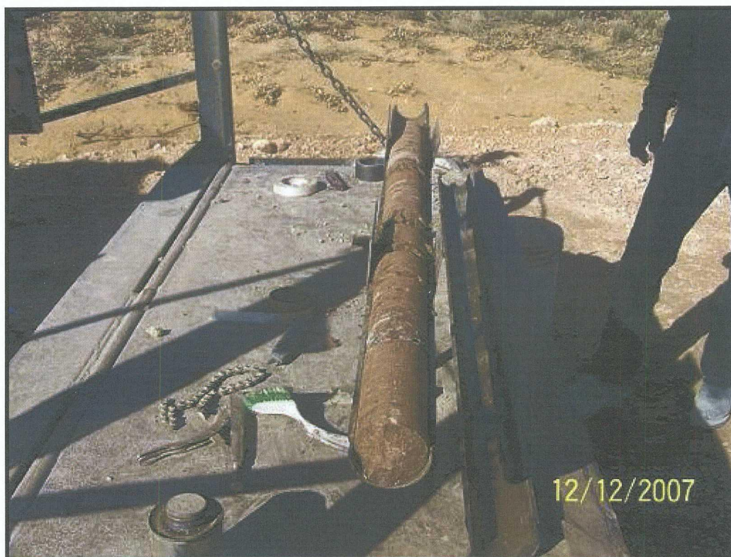
#22a- 138 to 142 feet. No break in core samples. Adjusted interval based on measured depth of borehole.
