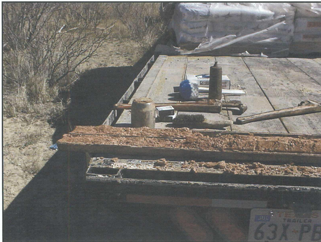
Figure 3. Example of five-foot core barrel sampling method (from an unrelated location)
