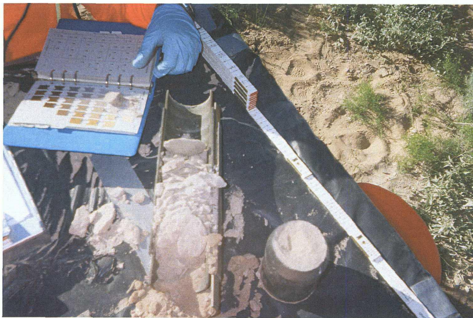
Photograph 14. Caliche sample from ring-sampler during the September 2006 geotechnical investigation.
