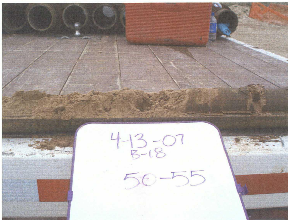
Photograph 18. Sand with very strong hydrocarbon odor and high PID readings (ranging from 1791 to 1,991 ppm) at South Site source area boring B-18/MW-7.
