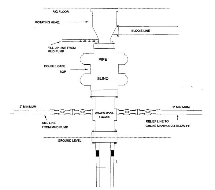
Minimum BOP installation for Completion operations. 7 1/16" Bore (6" Nominal), 3,000psi minimum working pressure double gate BOP to be equipped with blind and pipe rams.
