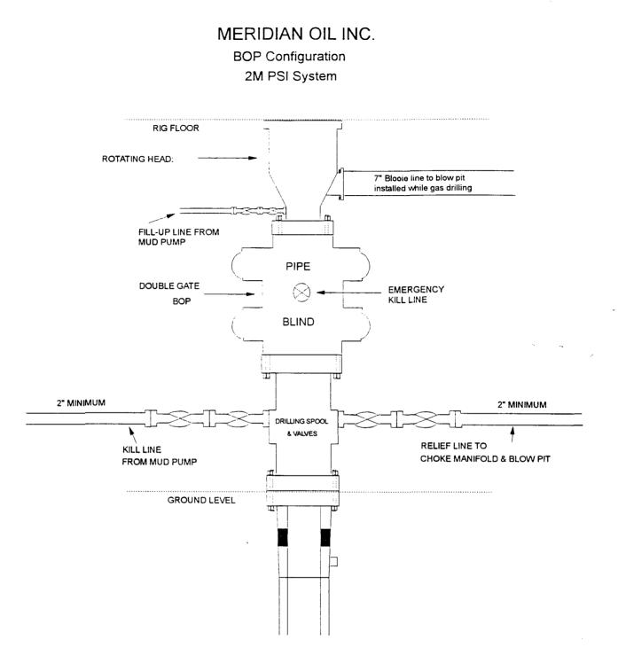
11" Bore, 3,000psi minimum working pressure double gate BOP to be equipped with blind and pipe rams. A Schaffer Type 50 or equivalent rotating head to be installed on the top of the BOP. All equipment is 3,000psi working pressure/or greater.
