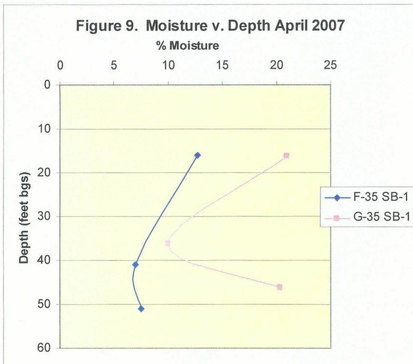
Higher soil moisture levels in the boring through the center of the excavation at G-35 than one similarly placed at F-35 may have been caused by storm water run-on at G-35. Whatever the cause, the vadose zone profile at G-35 is significantly wetter than F-35 and the data suggest that infiltration and flushing has effectively removed chloride from the vadose zone at G-35.
