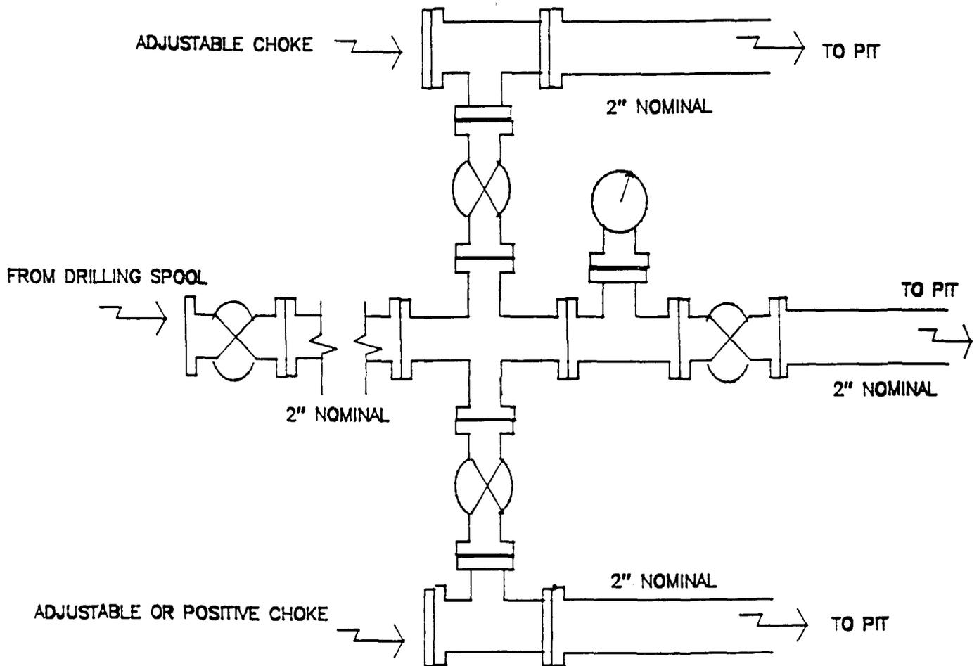
Minimum choke manifold installation from surface to Total Depth.
