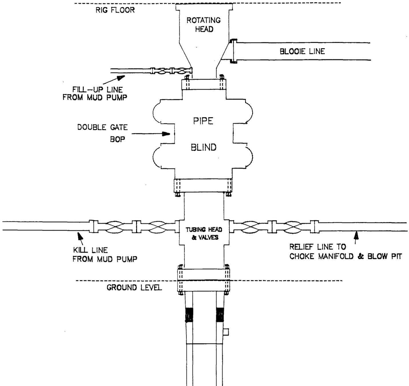
Minimum BOP installation for Completion operations. 7 1/16" Bore (6" Nominal), 3000psi minimum working pressure double gate BOP to be equipped with blind and pipe rams.
