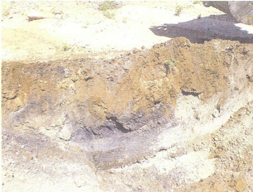
No 36 - This photo was taken of a north-south trench to a depth of 3 ft. in Section J. It shows the discolored soil conditions from 1-3 ft. along the trench wall.
