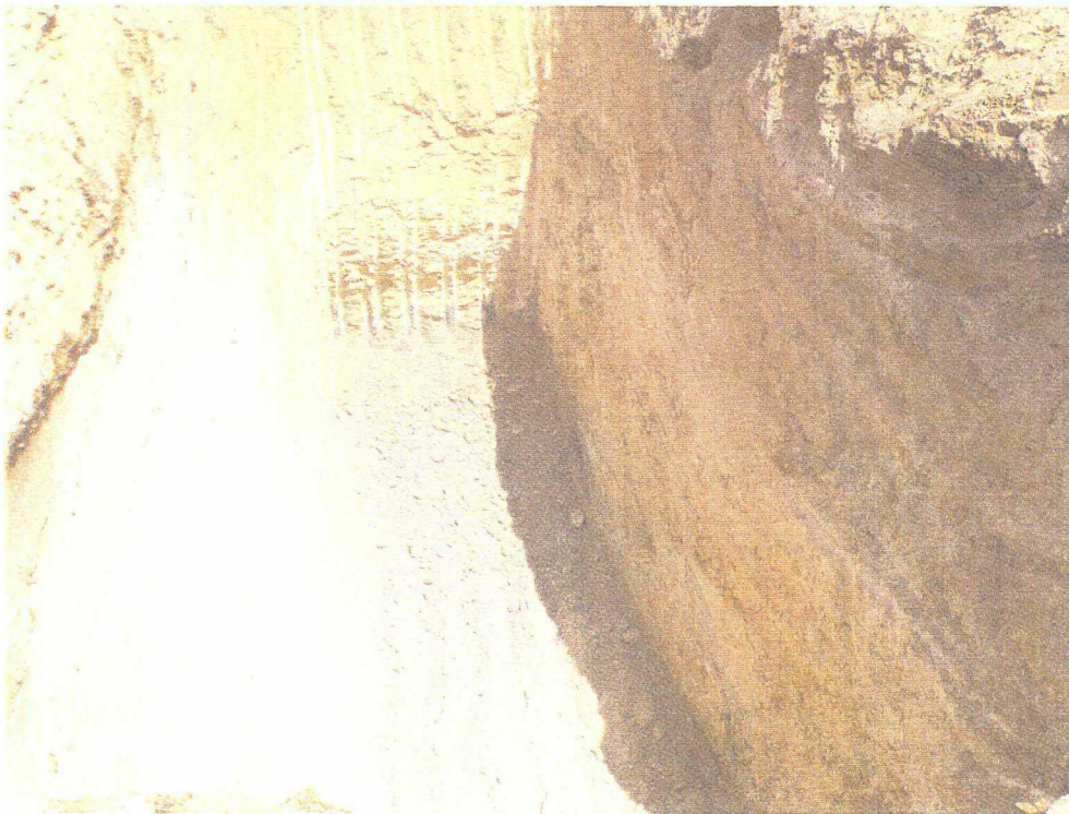
No 37 - This photo was taken at a test pit, centrally located at 500'E and 200'N. The pit was excavated with the track hoe to a depth of 14.5 ft. where refusal occurred. Discolored soils were encountered and can be seen at the bottom of the pit.
