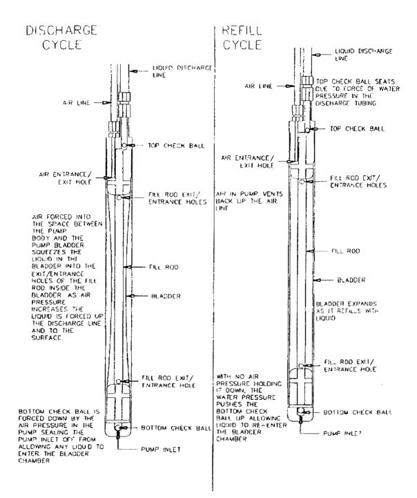
FIG. 4 Squeeze Type Bladder Pump
