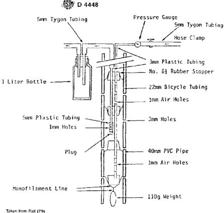
FIG. 7 Packer Pump Arrangement
