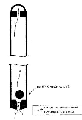
FIG. 2 Single Check Valve Bailer
