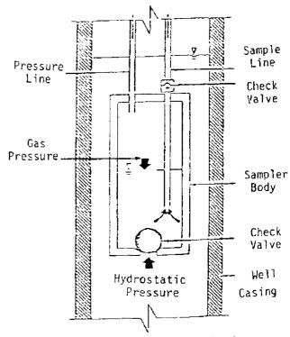
FIG. 5 The Principle of Gas Dispatcement Pumping
