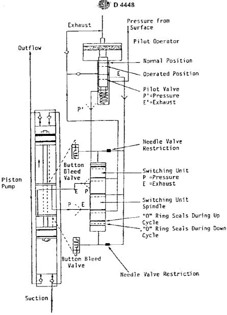
FIG. 6 Gas-Driven Piston Pump
