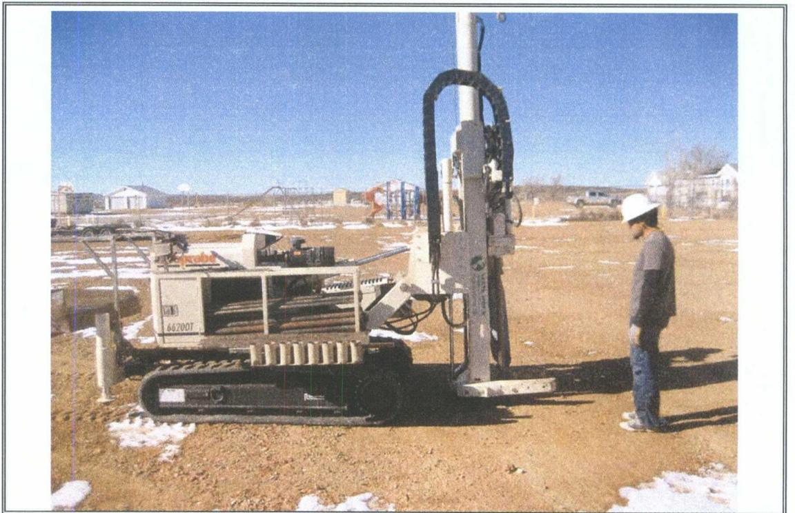
Photograph Number 18: View to the west of geo probe direct push unit performing soil borings
