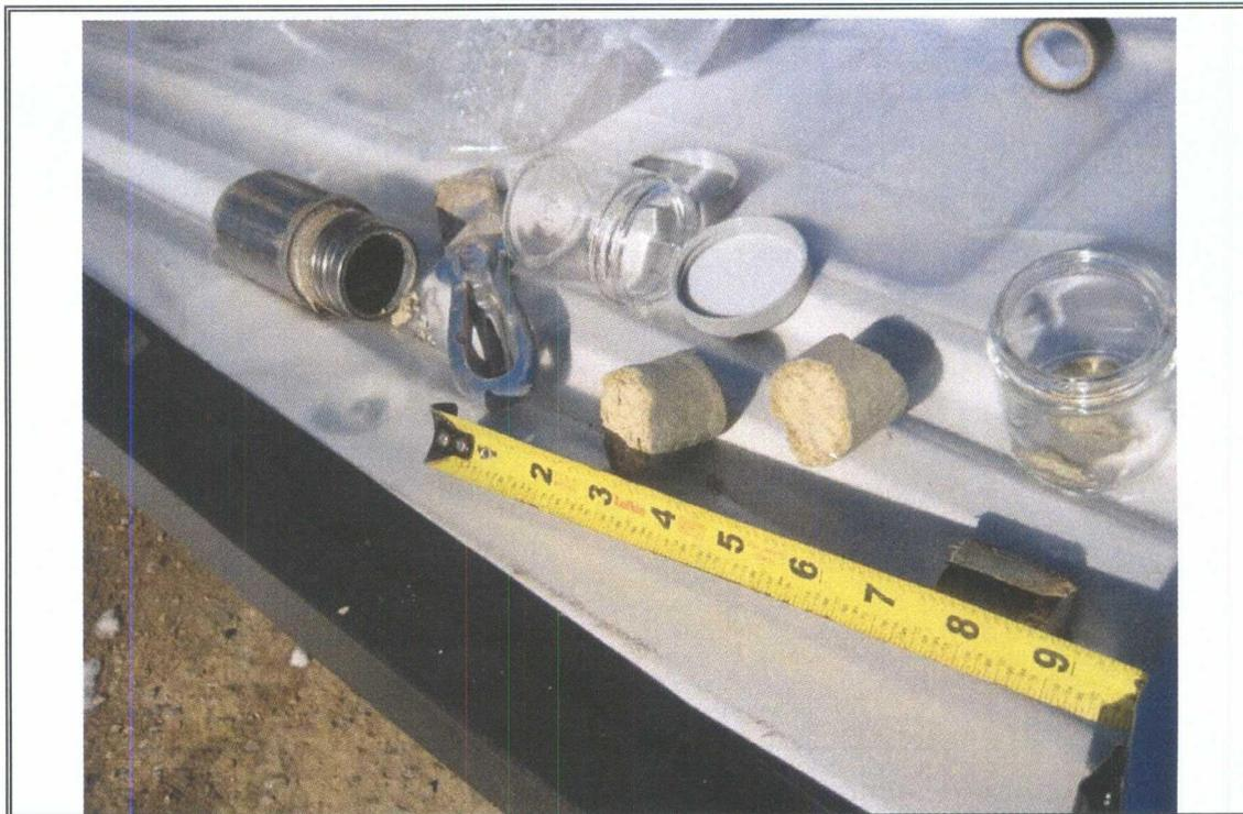
Photograph Number 19: View of sandstone encountered at approximately 17.5 feet below ground surface. The sand stone became harder at depth with geo probe refusal ranging from 17.5 to 21 feet below ground surface.
