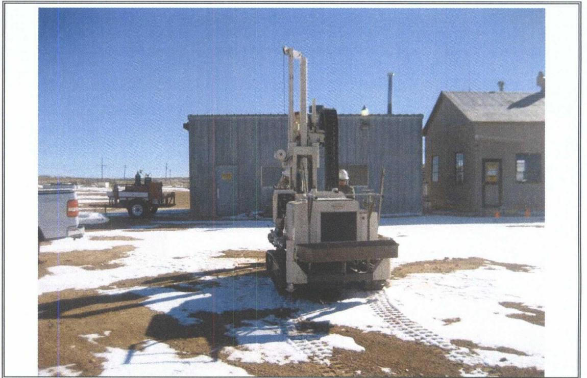
Photograph Number 15: View to the east of geo probe direct push unit performing soil borings
