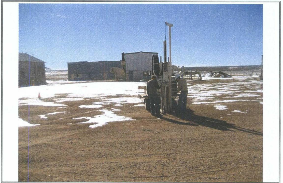
Photograph Number 17: View to the south of geo probe direct push unit performing soil borings.
