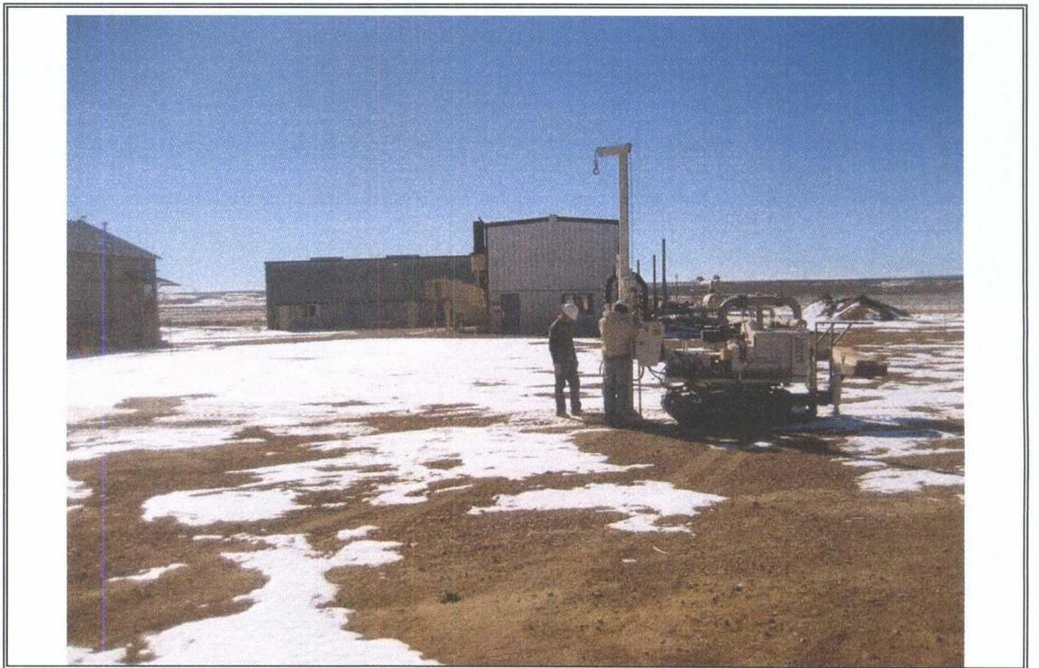
Photograph Number 16: View to the south of geo probe direct push unit performing soil borings.
