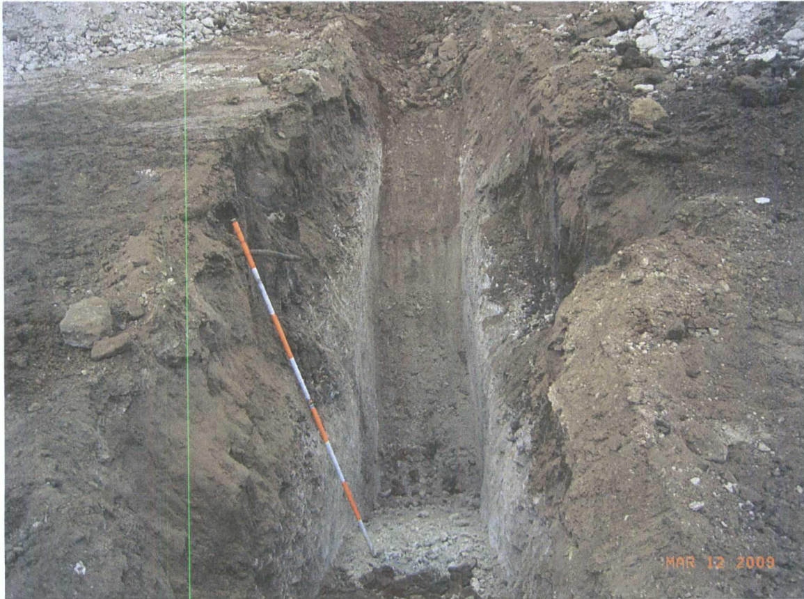
Exploration trench located near T-3. Soil staining (upper right on photo) has permeated the caliche. Yellow and grey zones of contamination (aromatics) were observed. Pit is aprox. 14 feet deep, sight rod is 8 feet high. 14 feet is the current dept the tracked excavator can dig.
