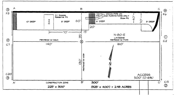
Reserve Pit Dike: to be 8' above Deep side (overflow + 3' wide and 1' above shallow side). Blow Pit: overflow pipe halfway between top and bottom and to extend over plastic liner and into plow pit
