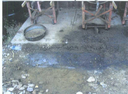
Photo 12: Discharge on ground near chemical dispensing area.
