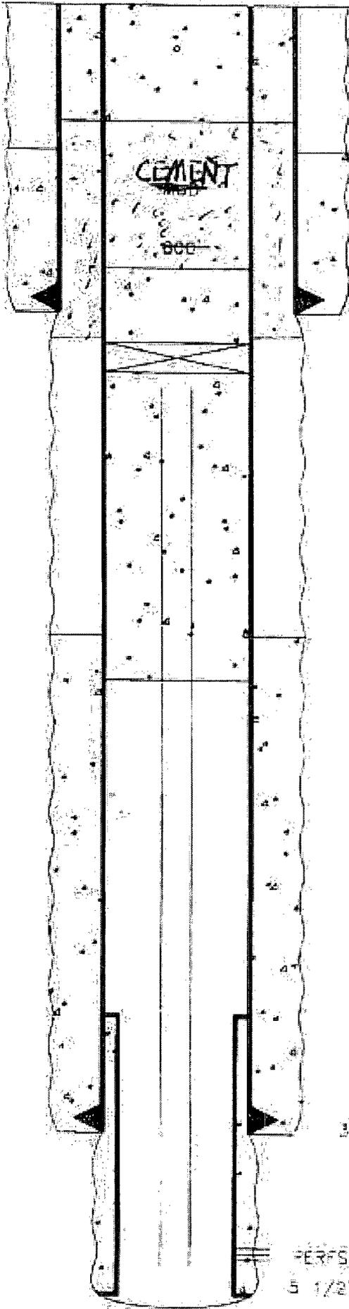
PERFORATE 7" @ <sup>980</sup> 300' CIRCULATE CEMENT TO SURFACE
