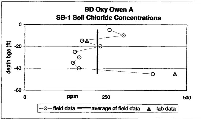
**Figure 2 – BD Oxy Owen A at/near source soil boring log with residual chloride and hydrocarbon concentrations.**
