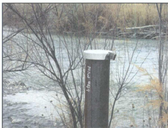
Padlock on MW #49 at River Terrace
