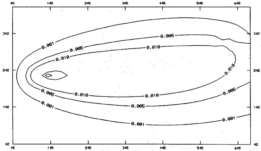
**Figure 7. Concentration contours for WinTran and SEFTRAN at the final time step for Test Case 5.**
