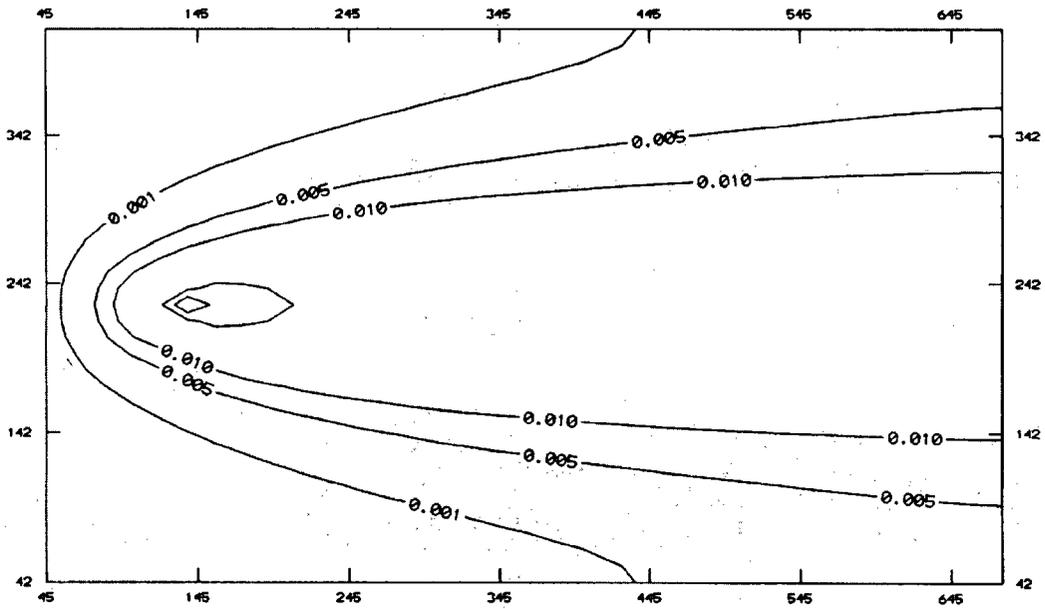
**Figure 4. Concentration contours for WinTran and SEFTRAN at the final time step for Test Case 2.**
