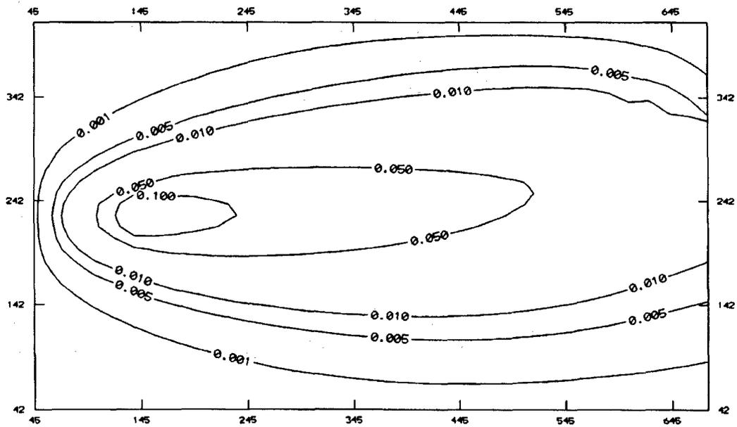
**Figure 8. Concentration contours for WinTran and SEFTRAN at the final time step for Test Case 6.**
