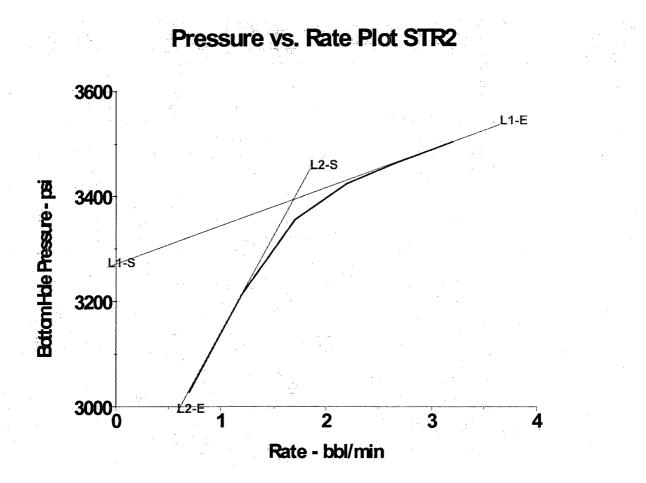
The second test illustrates the fracture parting pressure as 3394 psi.
