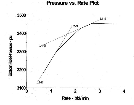
Lines L1-S & L2-S are based upon the inflection point of the rate vs. bottom hole pressure curve. The point of intersection defines the estimated fracture parting pressure, 3389 psi.
