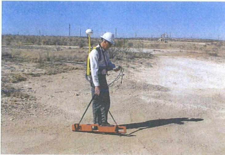
The EM-38 provides ground conductivity data at depths of 0-2.5' and 0-5' below ground surface. Here it is used to assess the impact of an historic brine water spill on the surface of an old production pad on BLM land.
