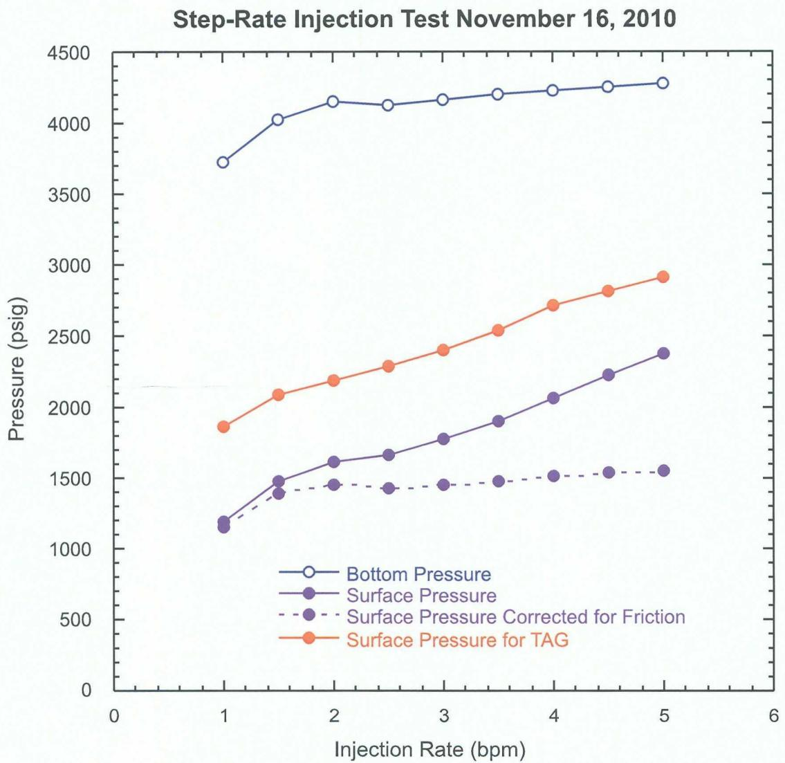
Figure 1: Results for the November 16, 2010 Step-Rate Test of the Pathfinder AGI #1. Hollow symbols correspond to bottom pressures and solid symbols correspond to surface injection pressures. The surface pressures have been corrected to remove friction (dashed line) and corrected to simulate TAG injection (red).
