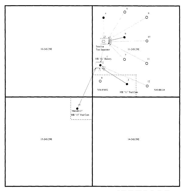
NOTE: Lines from wells to batteries denote only where wells are connected and the direction of flow, and do not indicate actual flowline routes.
