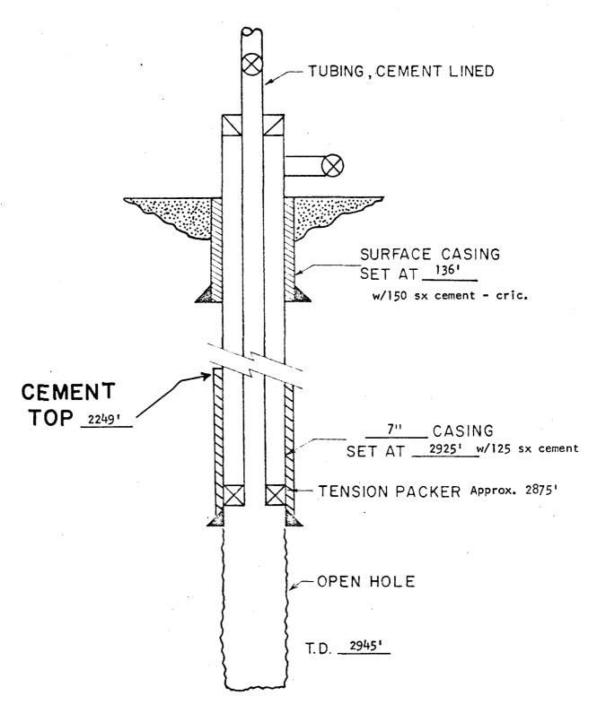
WATER INJECTION WELL SCHEMATIC
