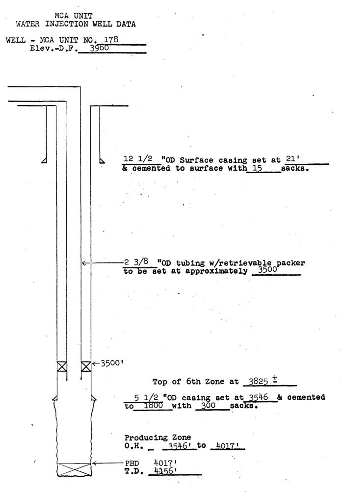
1) Clean out to 4017' 2) Connect up for water injection down the tubing as indicated.
