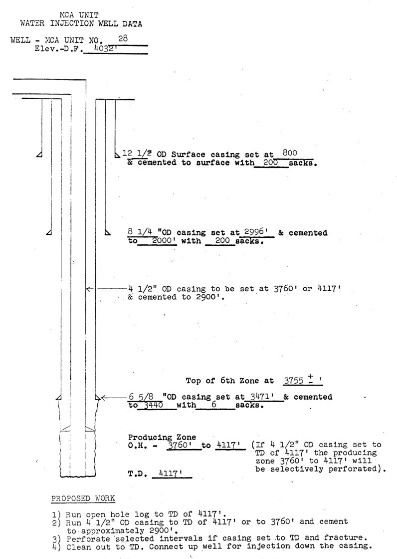
NOTE: The 6 5/8" OD casing may be cut & pulled.
