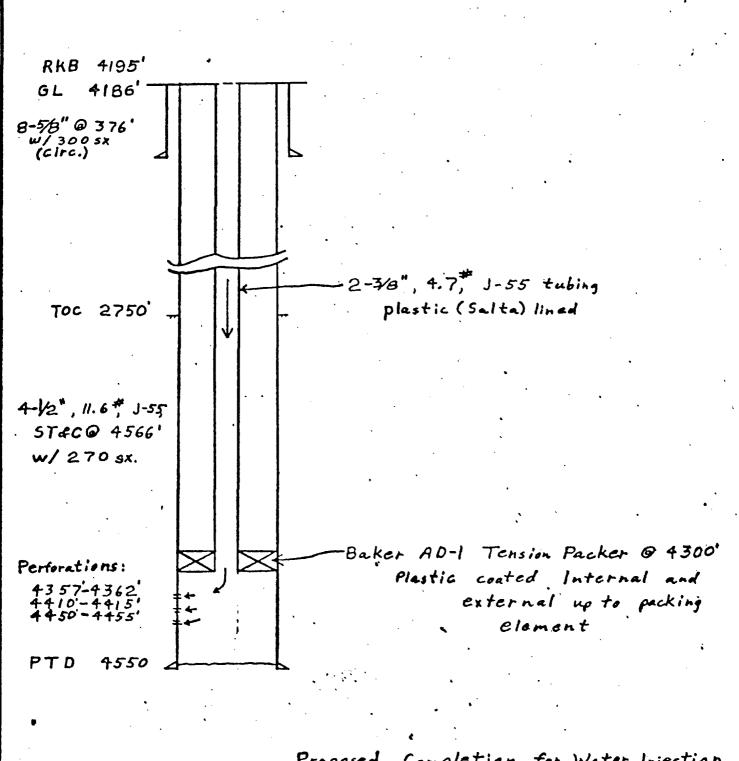
Proposed Completion for Water Injection
