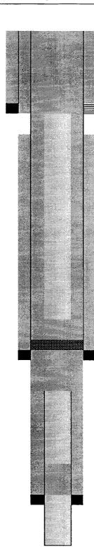
Perfd 9 5/8" csg at 255'. Circ 300 sx cmt to surf 9 5/8" x 16" csg annulus leaving 255' Cmt plug in top of 9 5/8" csg And 16" surf pipe.
