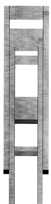
Perf'd 8 5/8" at 450'. Pumped 211 sx down 8 5/8" thru perfs At 450' and circulate.
