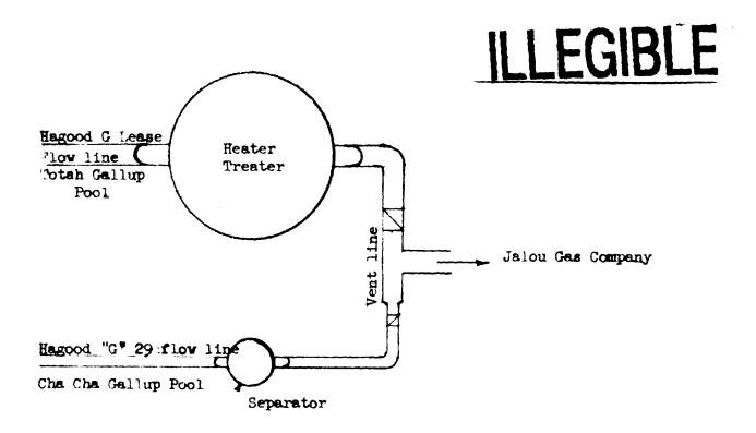
SCHEMATIC DIAGRAM Casinghead Gas Facilities Hagood "G" Well No. 29 Filliott, Inc.
