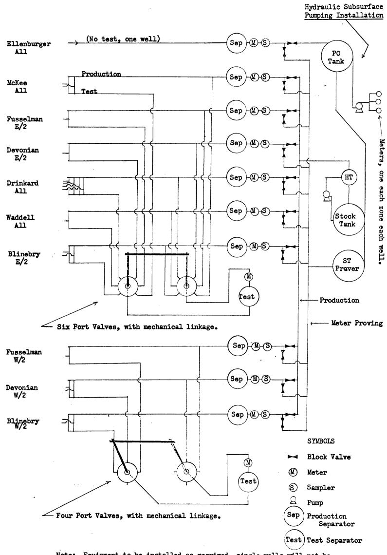
Note: Equipment to be installed as required, single wells will not be connected through test separators until a second well has been completed.
