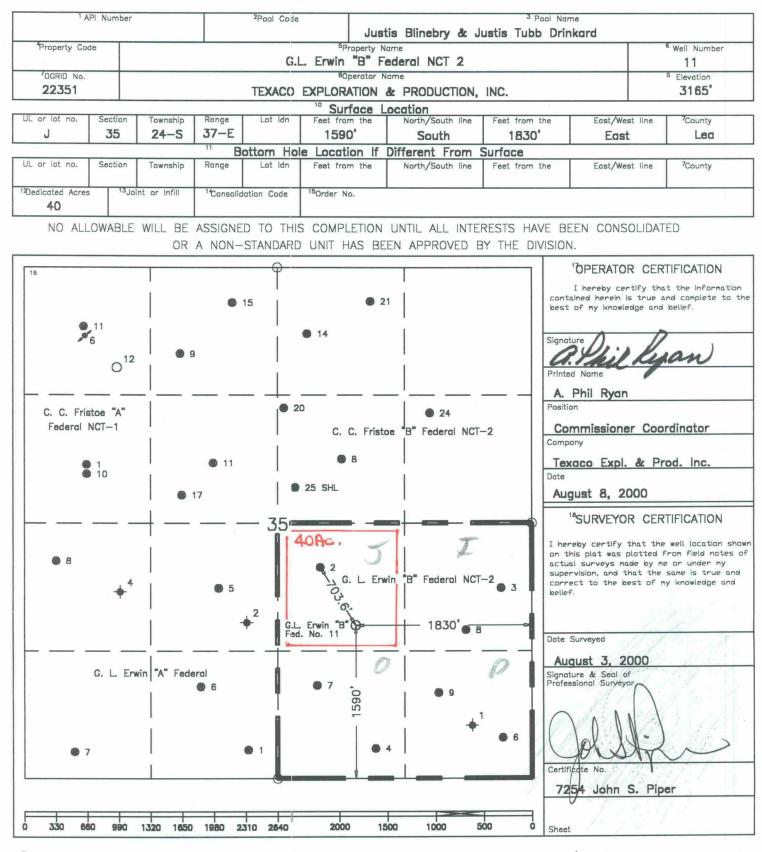
○ = Staked Location • = Producing Well ≠ = Injection Well • = Water Supply Well + = Plugged & Abandon Well ○ = Found Section Corner, 2 or 3" Iron Pipe & GLO B.C. ○ = Found /4 Section Corner, 1" Iron Pipe & GLO B.C.
