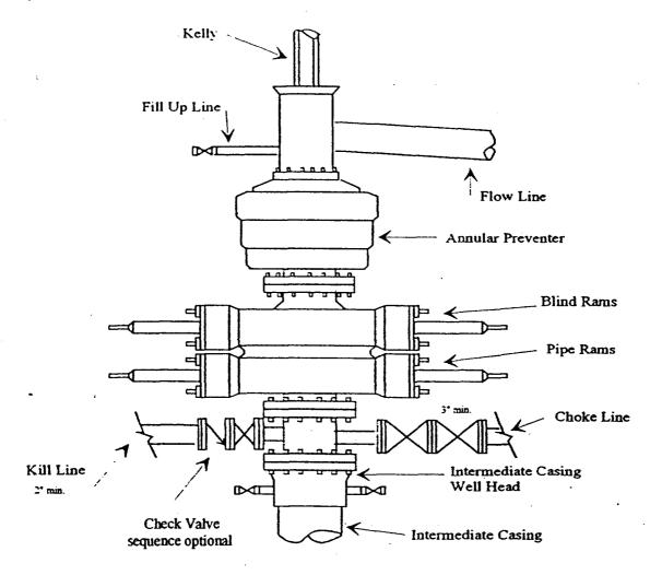
Typical 3,000 psi choke manifold assembly with at least these minimun features
