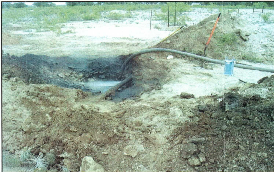
Produced water transportation line leak
