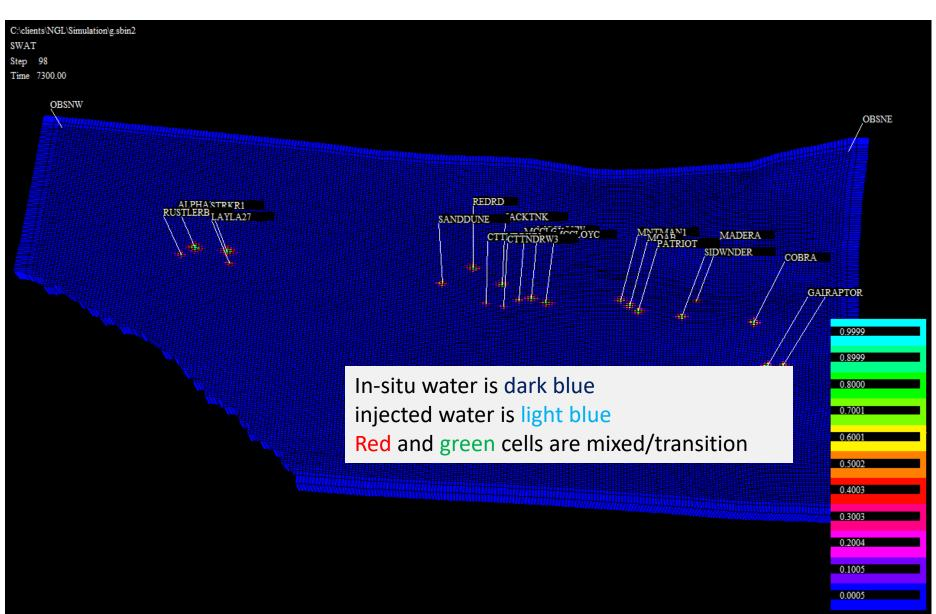
Detailed saturation profiles after 20 years of injection.
