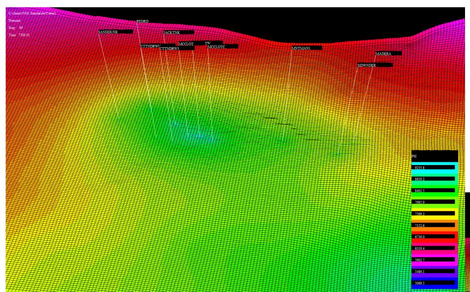
Large scale saturation profiles after 20 years of injection.
