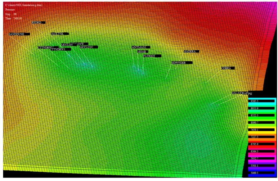
Pressure at 20 years is affected by original pressure, injected volumes, and the ability of the reservoir to dissipate pressure.
