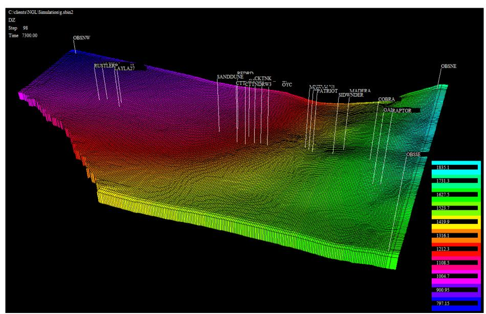
Initial pressure is equilibrated by the model based on grid cell depth, fluids(water) and capillary pressure.
