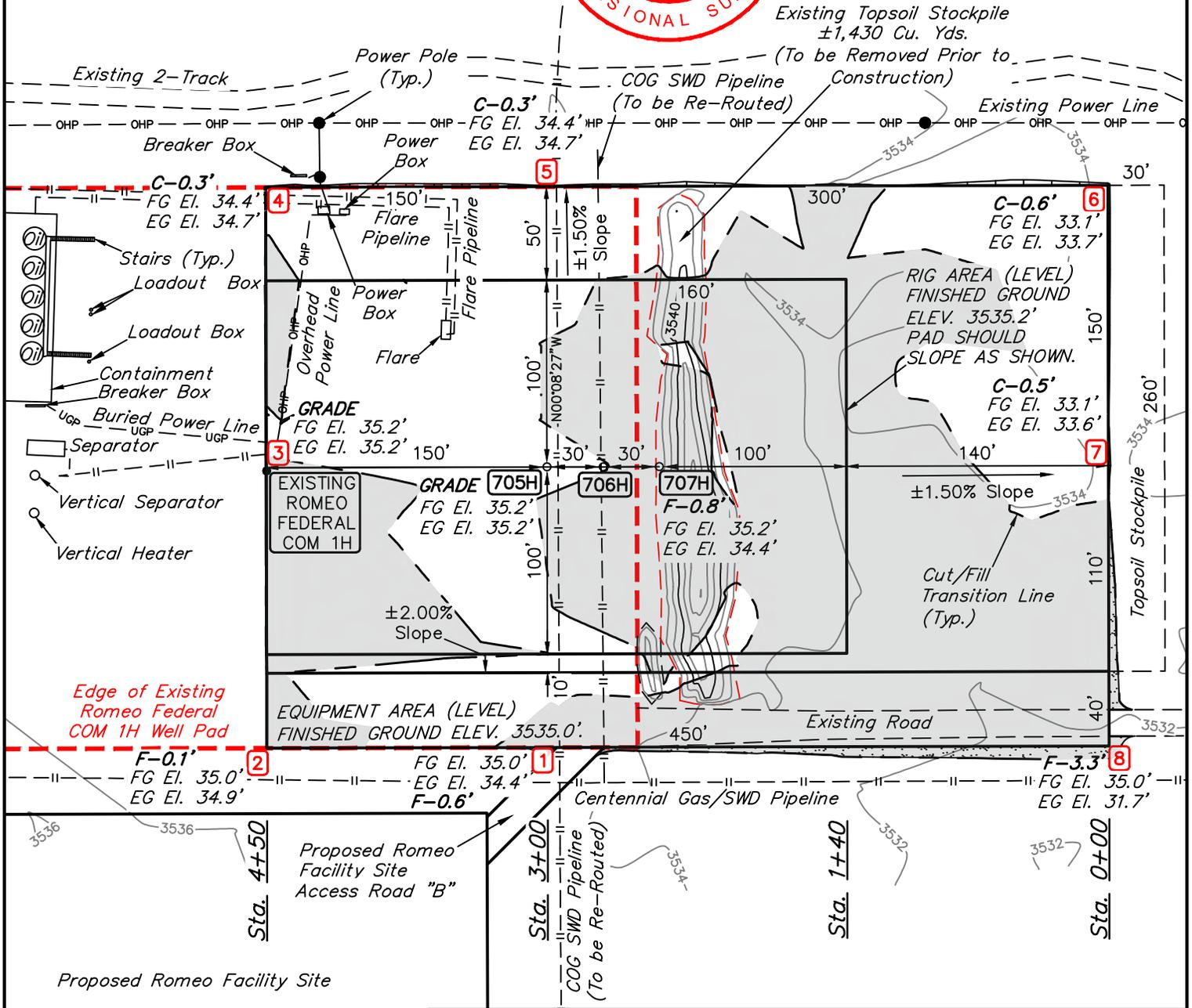
NOTE: Earthwork Calculations Require a Fill of 0.8' @ the 707H Location Stake For Balance. All Fill is to be Compacted to a Minimum of 95% of the Maximum Dry Density Obtained by AASHTO Method t-99.
