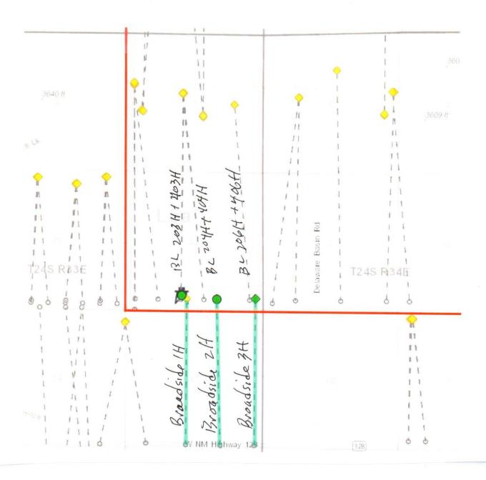
3. The proximity of the wellbores of the Broadside Wells to the wellbores of the Bell Lake Wells in Section 12 causes a serious potential collision risk. BC has apparently commenced drilling one of the Broadside Wells.
