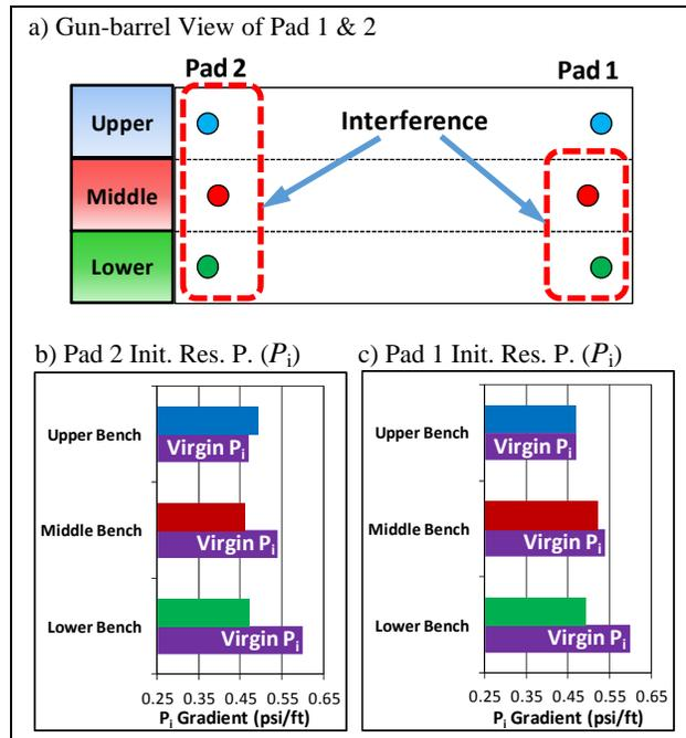
Figure 2: a) Gun Barrel View of Pad 1 and Pad 2 in stacked benches. b) Pad 2 initial reservoir pressures ( $P_i$ ) showing all three benches interfering. c) Pad 1 initial reservoir pressures ( $P_i$ ) showing **Middle & Lower** benches interfering.
