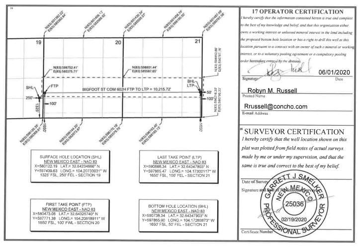
Bigfoot State Com #501H, #502H, #601H & #602H will be utilizing "lay down" laterals with Surface Hole Locations in Section 19, T19S-R28E with producing laterals in Sections 20 & 21, T19S-R28E, Lea County, NM.
